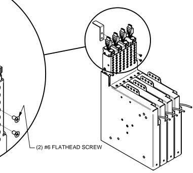
1b. FOR 3 OR FEWER RETRACTORS, INSTALL CHASSIS SUPPORT BRACKET ONTO RETRACTOR.
